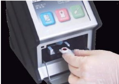
Insert the slide, press Anagnosis, input Cow ID and touch Start
